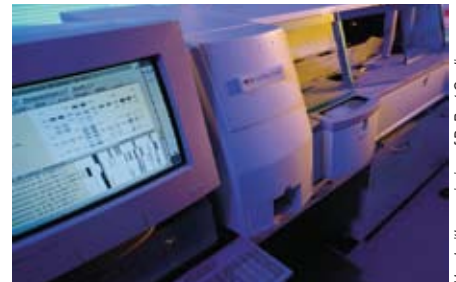
The automatic RiboPrinter® system from DuPont Qualicon identifies and characterizes bacteria through genetic "fingerprinting."
